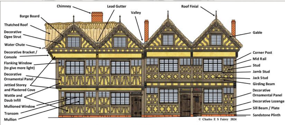
Diagram of the Conjectured Original Front Elevation of 46, 44 & 42 High Street (with Architectural Annotations)
