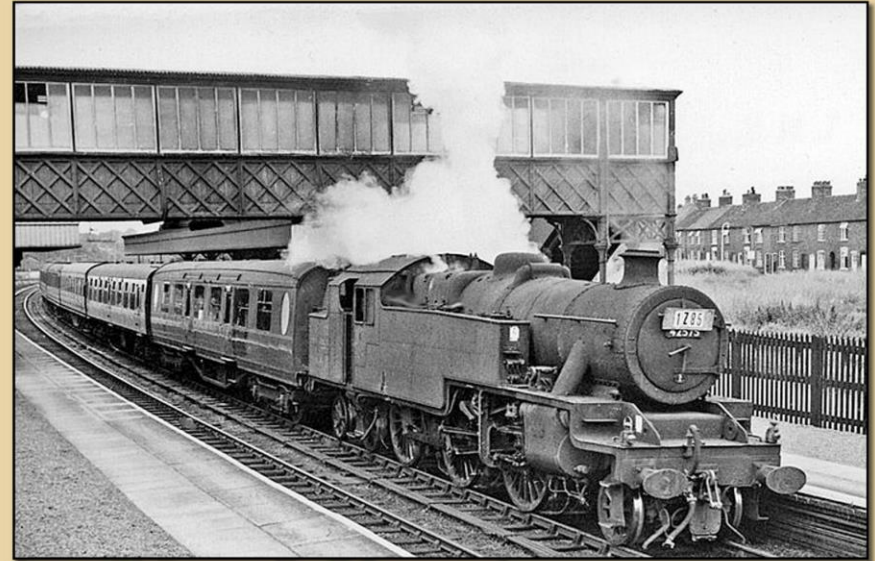
2-6-4T Stanier two-cylinder tank engine No 42575 heads an express special or excursion train southbound at Nantwich station.
